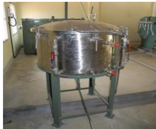
Centralised pressurised cocoon cooking unit
